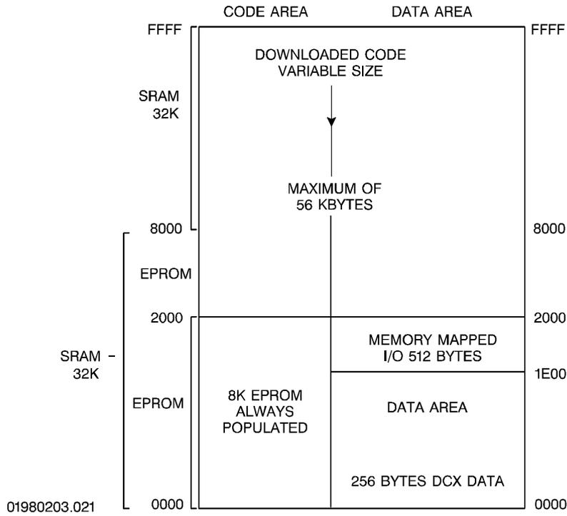
**SDC1 (16 KBytes EPROM 64 KBytes SRAM With Example NVRAM)**
