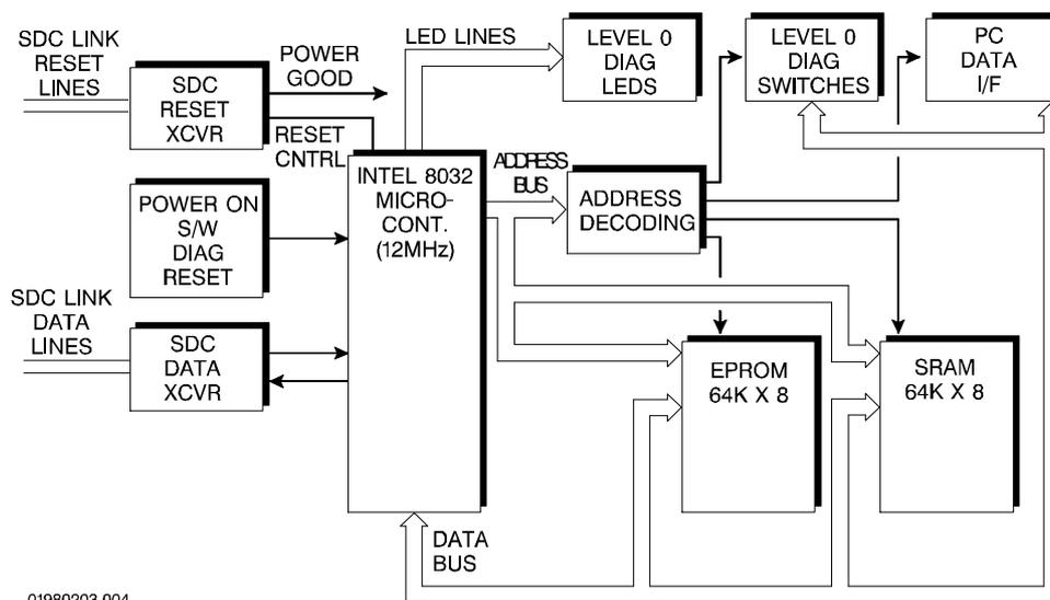
The SSPM houses the Serial Distributed Control (SDC) Master for the SDC link architecture. A master/slave scheme is implemented with each of the slaves being polled by the master.
