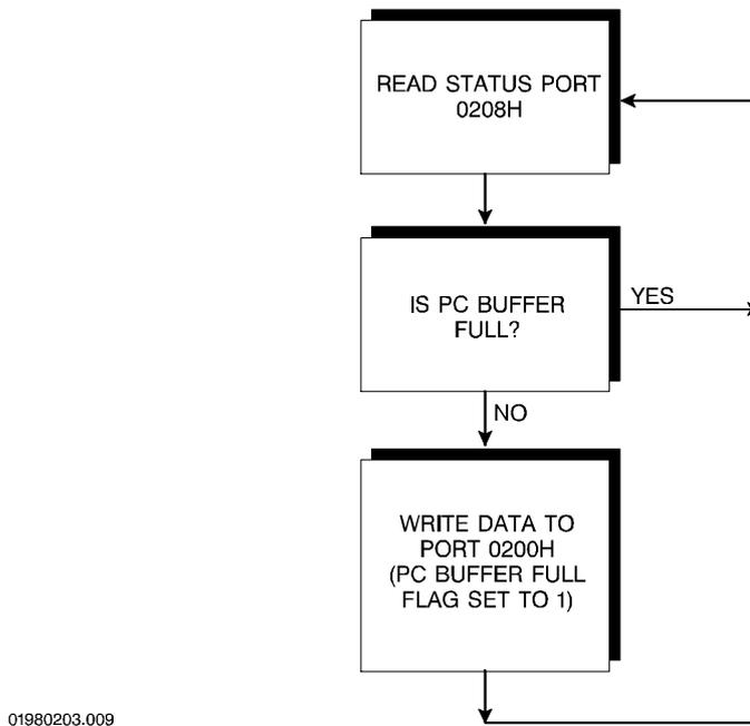
Writing data to PC\_DATA\_WR sets the PC\_BUFFER\_FULL flag to a "1" and also generates a PC\_BUFFER\_FULL interrupt to the SDC master.
