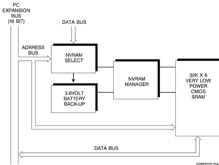
The SSPM provides a block of 32 KBytes of battery-backed RAM acting as System and Security Non-volatile RAM (NVRAM). (This is separate from NVRAM on the SDC master). The NVRAM is accessed from the PC Bus and appears in the PC's memory space in selectable areas from 0D0000H - 0DFFFFH.
