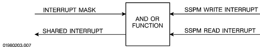
These are the flags SDC\_BUFFER\_FULL and PC\_BUFFER\_FULL (acting as an inverting PC\_BUFFER\_EMPTY flag). Thus an interrupt can be returned to the host PC when the SDC master writes data to it (a receive interrupt) or when the SDC master reads the data that the host PC had previously sent (a transmit interrupt).
