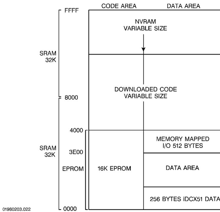
Optional NVRAM for State-Of-Health requirements is implemented as battery backed-up SRAM located from the top of data memory downwards. A small section of a battery-backed 32K SRAM is used for NVRAM. The amount used is specified as a base address at the top of NVRAM so that level 0 diagnostics will not overwrite the NVRAM on reset.
