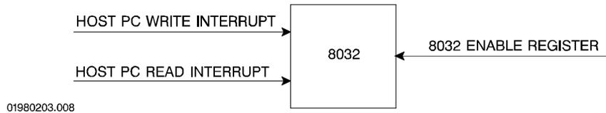
Both or either of the interrupt sources can be masked out by programming the 8032's Interrupt Enable register. In the case of an SDC\_BUFFER\_EMPTY (transmit) interrupt the cause of the interrupt will still be active until another byte is sent by the SDC master. Thus the interrupt should be disabled by the 8032 in the ISR until another byte is sent.
