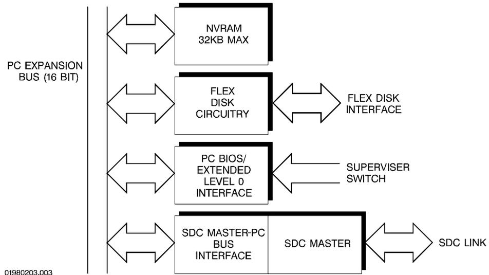
The SSPM printed circuit board operation is described under the following functional headings (refer to the schematic diagram for the SSPM, pages FO - 1 or FO - 9):
