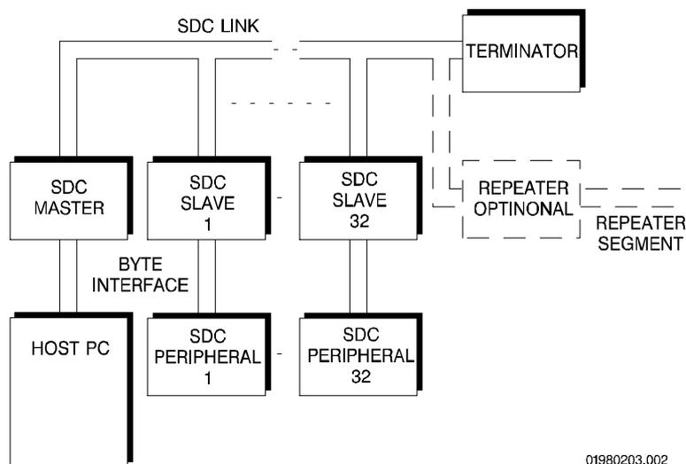
The SDC link is a serial multidrop link which permits the exchange of commands and data between a primary (master) node and a number of intelligent secondary (slave) nodes. Up to 32 physical devices may reside on the SDC link, each having one of 128 possible logical link addresses. The purpose of the link is to provide an expansion system:
